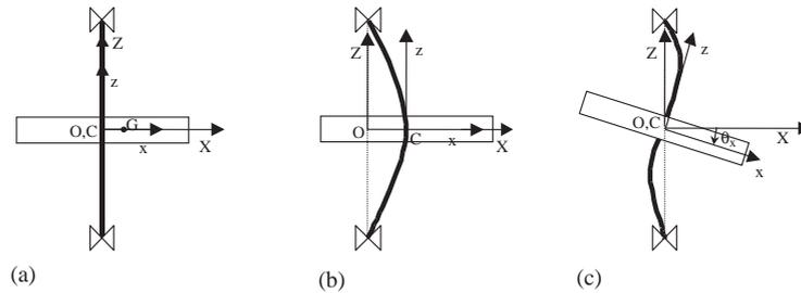
Fig. 1. The geometric setup and two vibration modes of the rotor system: (a) initial condition, (b) deflection motion, (c) inclination motion.
