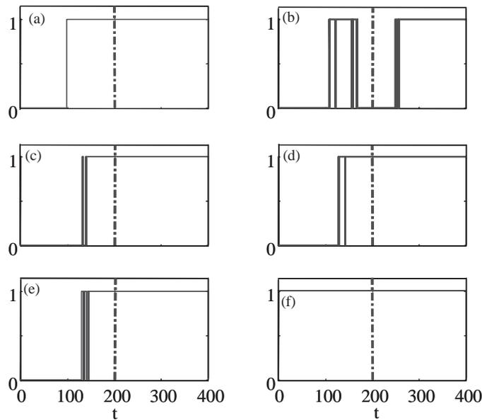
Fig. 5. The partial  $F$ -statistic tests for the model including all the effects. Zero means insignificant and one means significant. The dashed line is at  $t = 200$ . Each subfigure shows the test result for a specific factor: (a)  $\Delta'$ , (b)  $c'$ , (c)  $k'_{21}$ , (d)  $k'_{12}$ , (e)  $k'_{03}$ , (f)  $h'$ .
