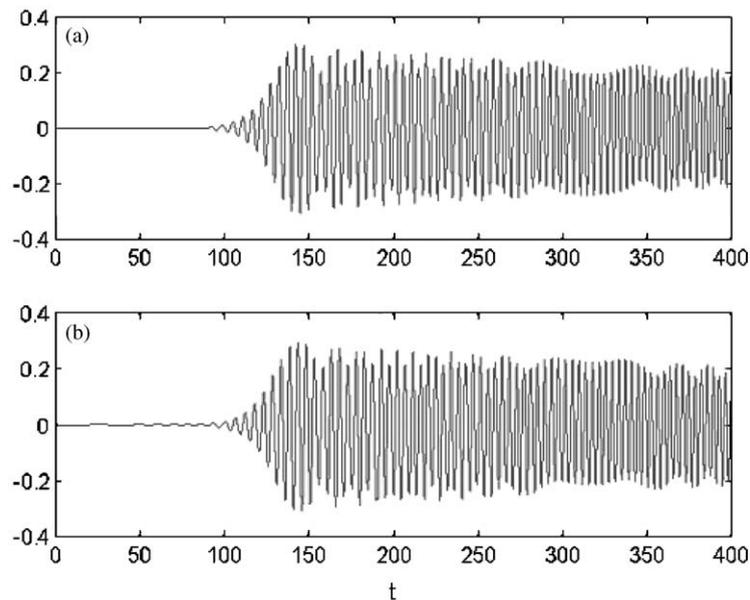
Fig. 3. The response of rotor during acceleration: (a)  $\theta_x$  and (b)  $\theta_y$ .
