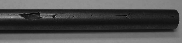
Fig. 2. An example of the image for the “checking” defect.
