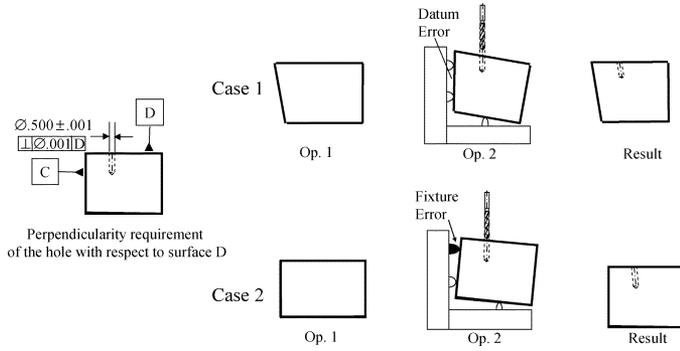
Fig. 1. Illustration of variation propagation.
