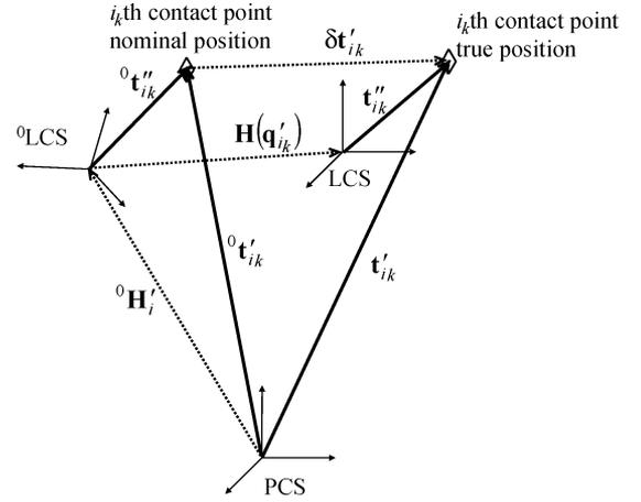
Fig. 7. Deviation of the  $i_k$ th contact point.
