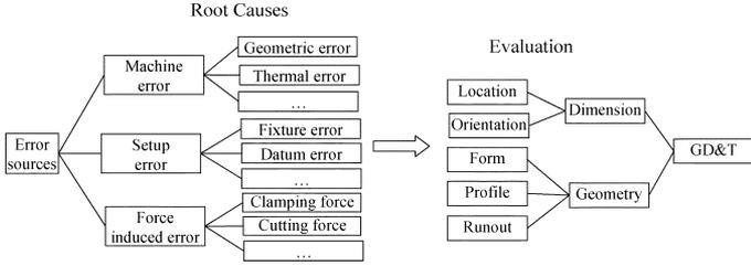
Fig. 2. Machining error sources and evaluation criteria.
