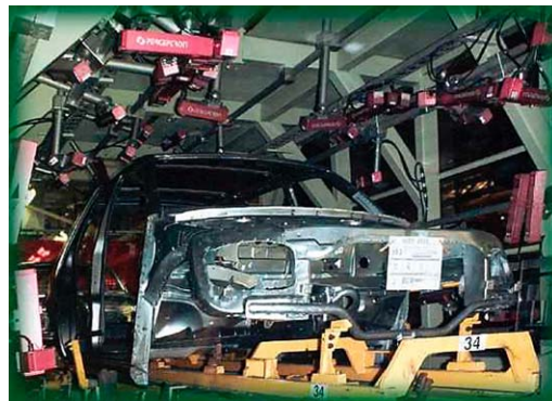
Figure 6. Automotive body at the optical measurement station.
